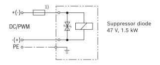
Recommended pre-fuse characteristics medium time-lag according to DIN 41571, 1.25 A.
