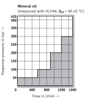
**Other approved hydraulic fluids** (see page 5) (simulated; kinetic viscosity 40 mm<sup>2</sup>/s)
