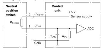
$$U_{\text{OUT}} = \frac{U_{\text{Supply}} \times R_{\text{PD}}}{R_{\text{PD}} + R_{\text{Sensor}}}$$
