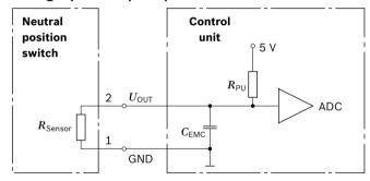
$$U_{\text{OUT}} = \frac{U_{\text{Supply}} \times R_{\text{Sensor}}}{R_{\text{PU}} + R_{\text{Sensor}}}$$
