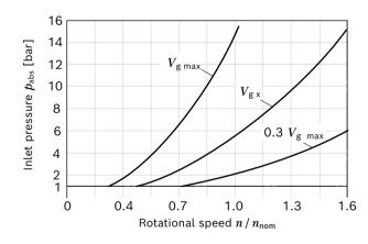
This diagram is only valid for the optimum viscosity range of  $\nu_{opt}$  = 36 to 16  $mm^2/s.$
