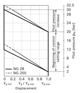
10 **A6VE Series 63** | Variable plug-in motor HD – Proportional control, hydraulic
