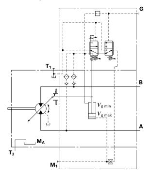
14 **A6VE Series 63** | Variable plug-in motor EP – Proportional control, electric
