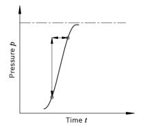
Maximum differential pressure at the shaft seal
