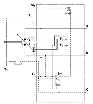
18 **A6VE Series 63** | Variable plug-in motor HA – Automatic control, high-pressure related
