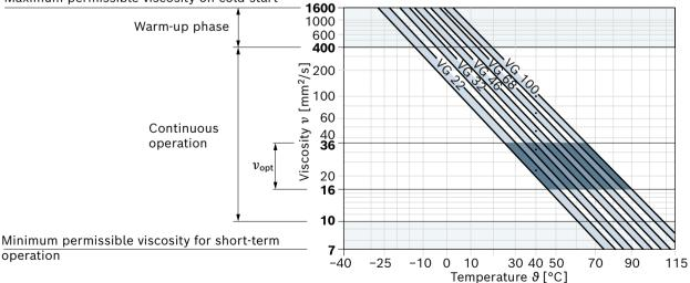
1) This corresponds, for example on the VG 46, to a temperature range of +4  $^{\circ}\mathrm{C}$  to +85  $^{\circ}\mathrm{C}$  (see selection diagram)
