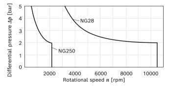
Minimum pressure – operation as a pump (inlet)
