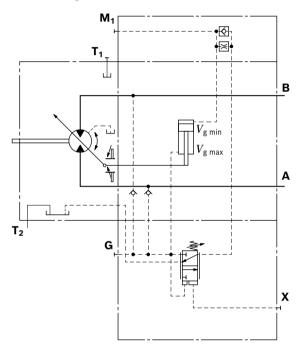
20 **A6VE Series 63** | Variable plug-in motor HA – Automatic control, high-pressure related
