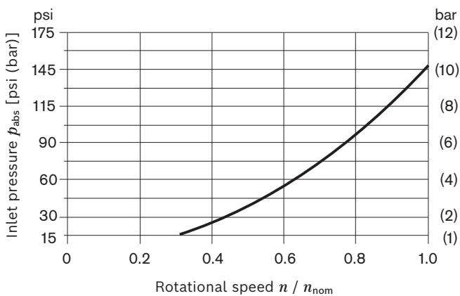
This diagram is only valid for the optimum viscosity range of  $\nu_{\text{opt}} = 170$  to 73 SUS (36 to 16 mm<sup>2</sup>/s).
