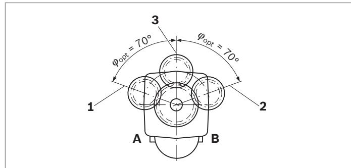
1 "Counter-clockwise" rotation. Pressure at port B
