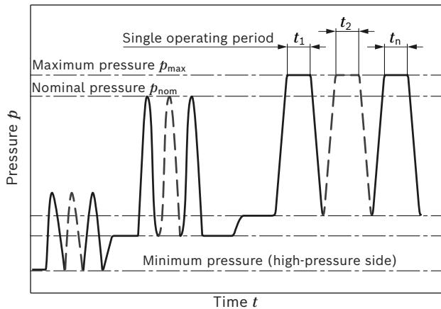
Total operating period =  $t_1 + t_2 + \dots + t_n$
