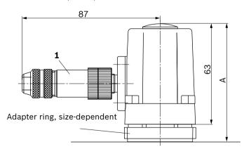
1 Plug-in connector is included in the scope of delivery.
