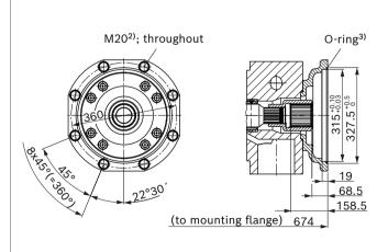
1) Mounting holes pattern viewed on through drive with control at top
