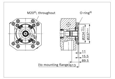
1) Mounting holes pattern viewed on through drive with control at top
