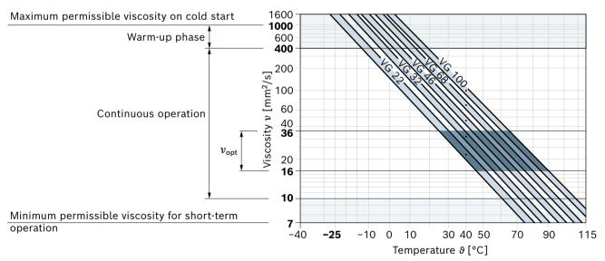
This corresponds, for example on VG 46, to a temperature range of +4 °C to +85 °C (see selection diagram)2)
