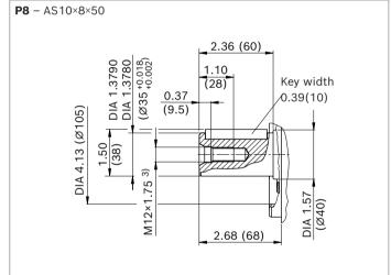
ANSI B92.1a, 30° pressure angle, flat root, side fit, tolerance class 5
