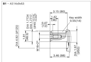
$_{\rm 1)}$  ANSI B92.1a,  $30^{\rm o}$  pressure angle, flat root, side fit, tolerance class 5
